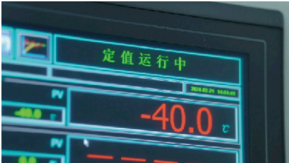
HMI display Low-temperature performance test under -40°C
