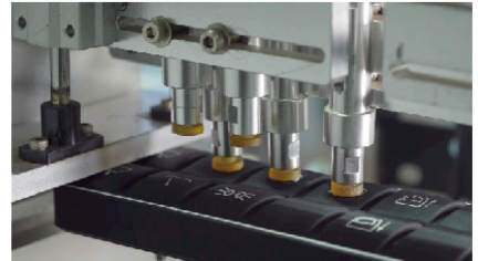
Panel buttons 1.2 million times reliability test
