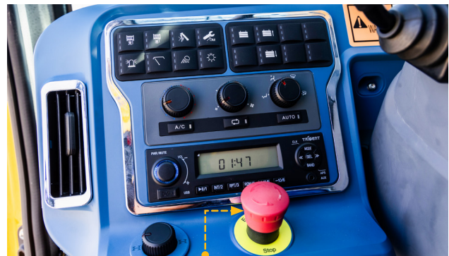
Superstructure emergency stop switch
