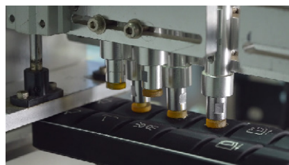
Panel buttons 1.2 million times reliability test
