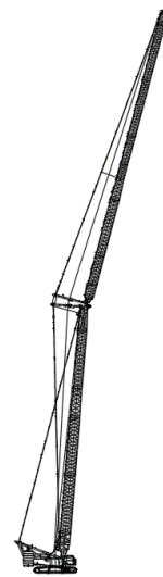
Operation mode of tower jib (HW)
