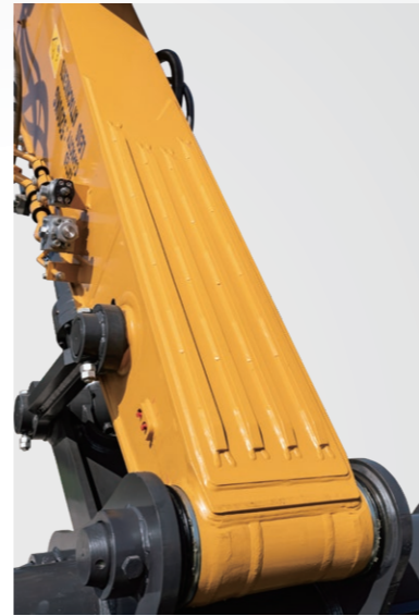
Specially designed long strengthened strike beams installed to prevent damage to dipper arm.
