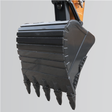
Reinforced rock bucket and teeth
